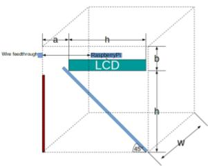
The dimensions of the box are derived from the Monitor. It is important the some depth (a) is added to the box compared to the distance between bottom and LCD (h). This distance will be the precived distance between background and projection.
