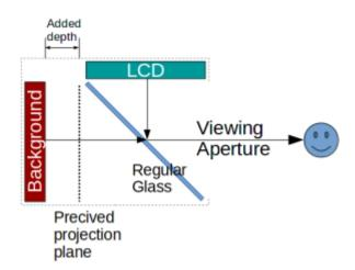
By choosing the box dimensions right, the light path from the background to the viewer is made longer than the path from the LCD. The projection is thus precived as freestanding in front of the background instead of on it. This causes two 2D layers to be precived as a 3D scene.
