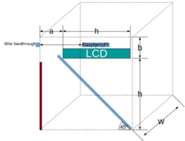
The dimensions of the box are derived from the monitor. It is important that some depth (a) is added to the box compared to the distance between bottom and LCD (h). This distance will be the perceived distance between background and projection.
