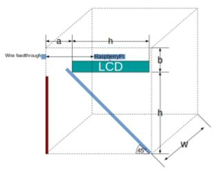
The dimensions of the box are derived from the monitor. It is important that some depth (a) is added to the box compared to the distance between bottom and LCD (h). This distance will be the precived distance between background and projection.
