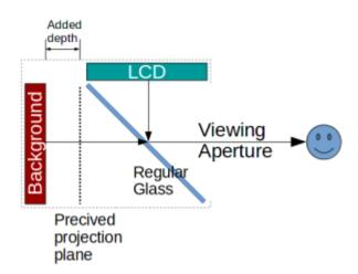
By choosing the box dimensions right, the light path from the background to the viewer is made longer than the path from the LCD. The projection is thus precived as freestanding in front of the background instead of on it. This causes two 2D layers to be precived as a 3D scene.
