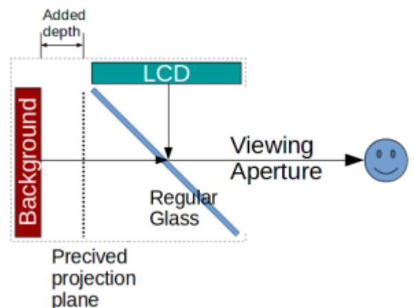
By choosing the box dimensions right, the light path from the background to the viewer is made longer than the path from the LCD. The projection is thus perceived as freestanding in front of the background instead of on it. This causes two 2D layers to be perceived as a 3D scene.
