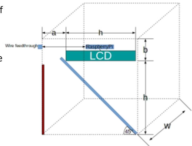
The dimensions of the box are derived from the Monitor. It is important the some depth (a) is added to the box compared to the distance between bottom and LCD (h). This distance will be the precived distance between background and projection.
