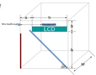
The dimensions of the box are derived from the monitor. It is important that some depth (a) is added to the box compared to the distance between bottom and LCD (h). This distance will be the precived distance between background and projection.
