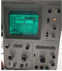
This works with both raster and pure vector mode. The Image on the right is made using raster mode.
