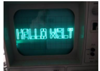
The solution comes from the other digital to analog converter still commonly found on modern PCs: The VGA-Port. While it may be intended to drive raster screens, it essentially is a 3 Channel, High-speed (> 100MHz) DAC. Using 2 of these channels (Red and Green) the electron beam of an Oscilloscope can be driven in X and Y directions much like the soundcard method, but much faster and without the harmful filter stages. This makes it almost ideal for drawing vector graphics on a scope.
