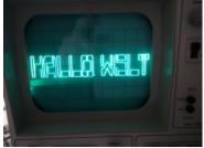
The solution comes from the other digital to analog converter still commonly found on modern PCs: The VGA-Port. While it may be intended to drive raster screens, it essentially a 3 Channel, High-speed (> 100MHz) DAC. Using 2 of these channels (Red and Green) the electron beam of an Oscolloscop can be driven in X and Y directions much like the soundcard method, but much faster and without the harmful filter stages. This makes it almost ideal for drawing vector graphics on a scope.
