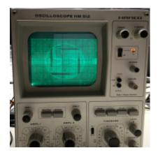
The trick of changing the brightness of vector paths can be used to display raster images.
