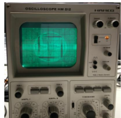
The trick of changing the brightness of vector paths can be used to display raster images.
