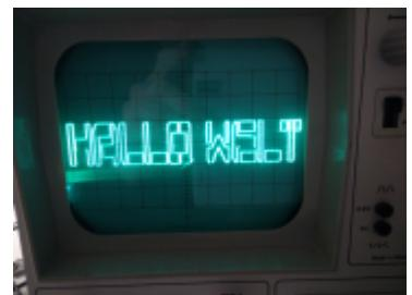
The solution comes from the other digital to analog converter still commonly found on modern PCs: The VGA-Port. While it may be intended to drive raster screens, it is essentially a 3 Channel, High-speed (> 100MHz) DAC. Using 2 of these channels (Red and Green) the electron beam of an Oscilloscope can be driven in X and Y directions much like the soundcard method, but much faster and without the harmful filter stages. This makes it almost ideal for drawing vector graphics on a scope.
